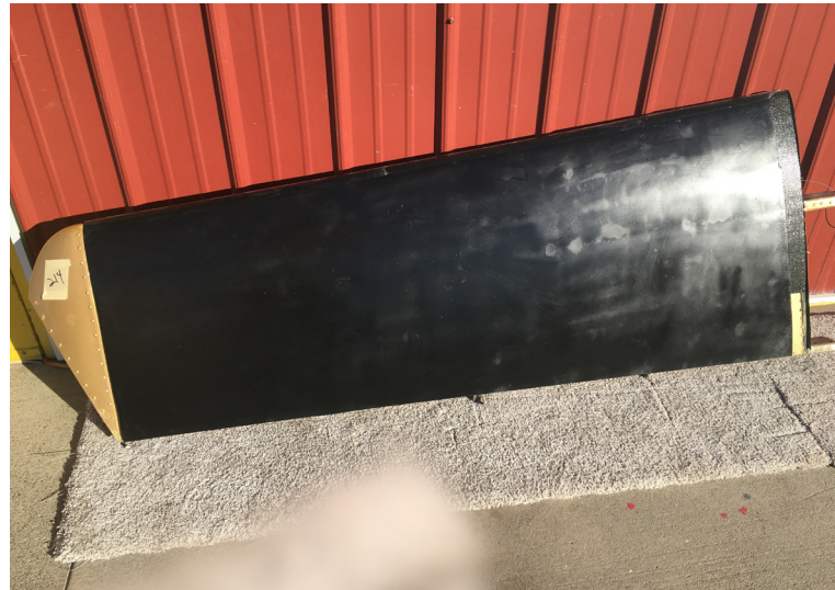
CARBON FIBER FLIGHT CONTROL SURFACES AUTOCLAVED @350°F/100PSI
