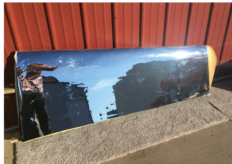
CARBON FIBER FLIGHT CONTROL SURFACES AUTOCLAVED @350°F/100PSI
