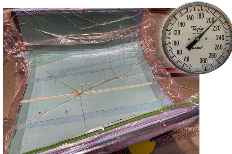
CARBON FIBER/CERAMIC UPPER COWLING VACUUM BAGGED, OVEN CURED at 210° F
