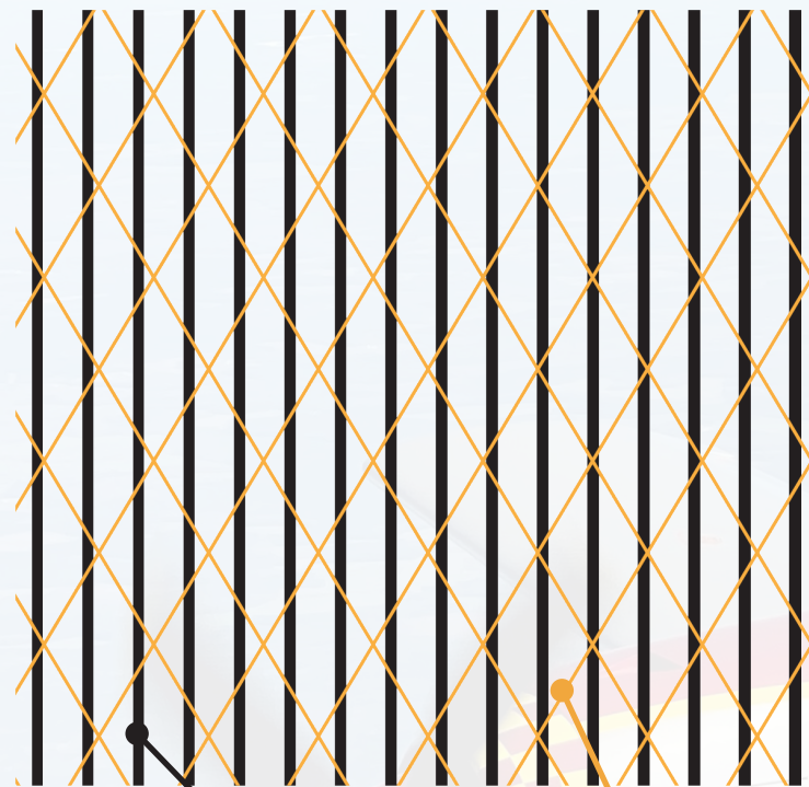
CARBON FIBER TOW 90° ZOLON TOW ± 45° FSU (FIBER SCRIM-BACK UNIT)
