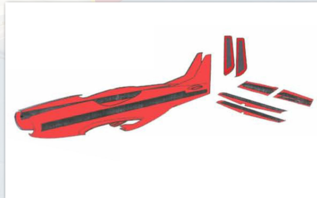
Spar and Longeron Molds
